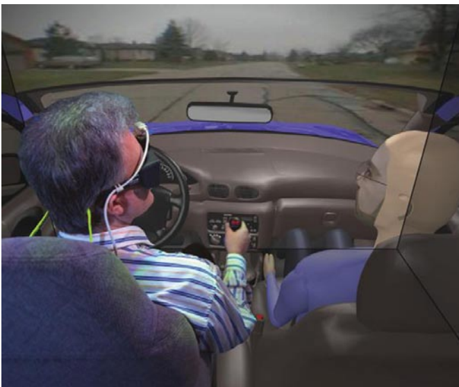
Above: VisualEyes, a tele-immersive method for long-distance collaboration work on car interior development. Two people sit in a virtual rendering of a possible car interior, which can be updated by a 3D modeling technician based on the suggestions of the developers.
